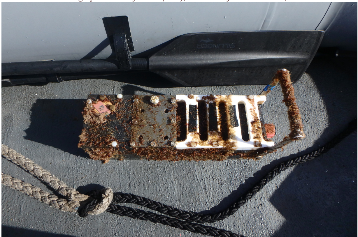
The PCO 2 CARIOCA sensor located at 10 m depth on the BOUSSOLE buoy after its recovery by divers.
